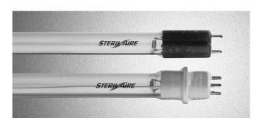
Steril-Aire's shatter-resistant UVC Emitters are ideal for use in critical applications found in the food, beverage and life science industries. Steril-Aire UVC Emitters are coated with a protective plastic sleeve from end to end. If dropped or broken, glass fragments and mercury remain safely contained. The sleeving is also designed to prevent moisture intrusion for use in wash down areas.
